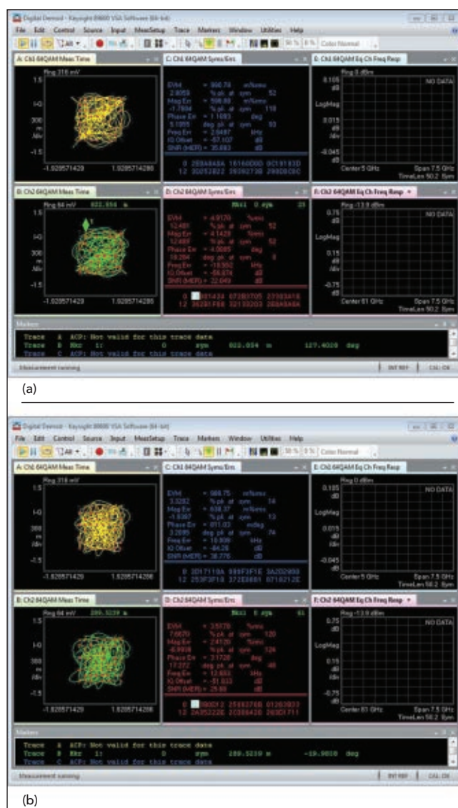
▲ Fig. 5 EVM performance without DPD (a) and with DPD (b).
