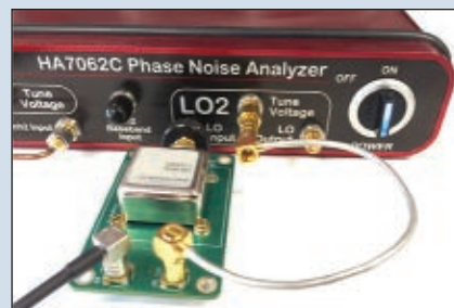
▲ Fig. 2 The external LO mode function was developed primarily for evaluating crystal oscillators.
