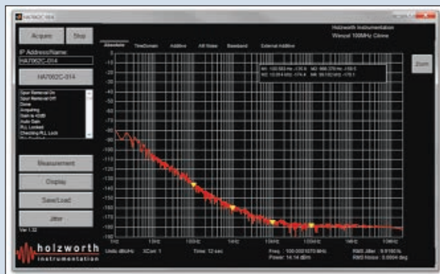
▲ Fig. 6 GUI screenshot showing the phase noise measurement of a 100 MHz OCXO, down to a 1 Hz offset.
