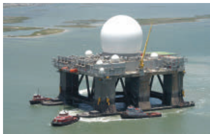
▲ Fig. 7 SBX-1 sea-based X-Band phased-array radar. Source: U.S. Navy Military Sealift Command.
